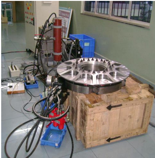
Hydraulic Multicylinder for Aircraft Arrestor Braking Systems designed and built inhouse
